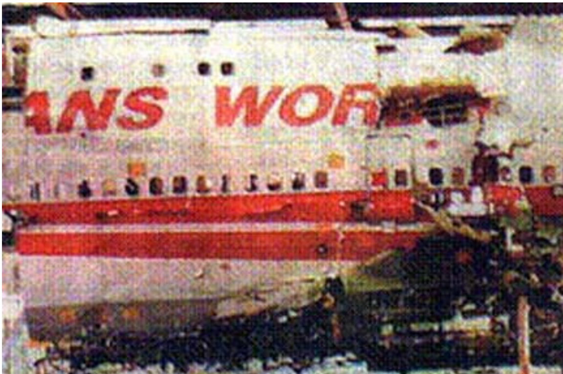
Caption for above photograph: Photograph of the port side of Trans World Airlines Flight 800 showing the relative undamaged skin forward of the wing.
