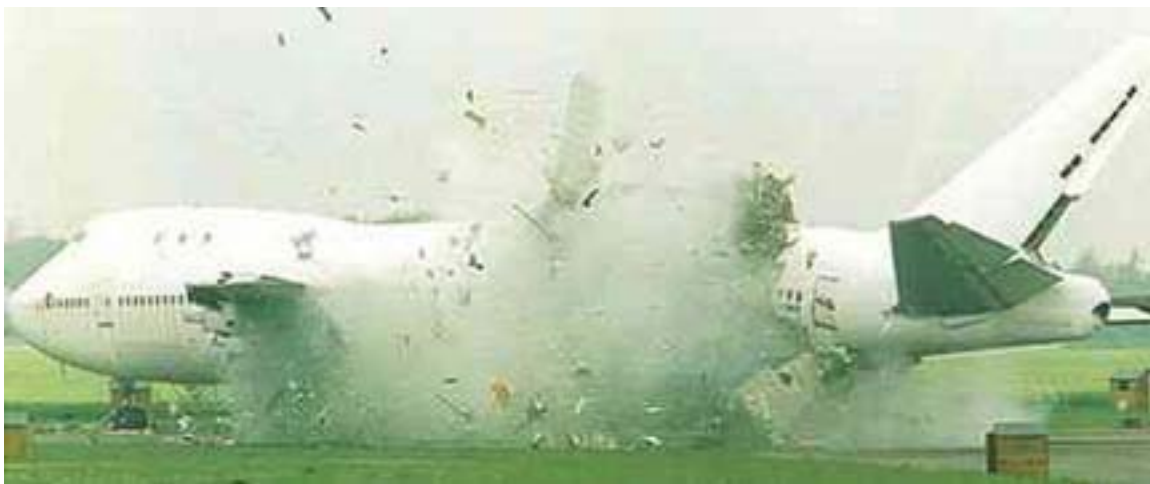
Caption for above photograph: Staged bombing of a Boeing 747 at Bruntingthorpe UK showing the massive damage which occurs when a real bomb goes on in a Boeing 747.
