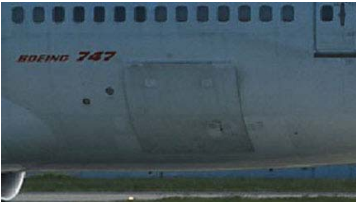
Caption for above photograph: Closeup of Boeing 747 closed forward cargo door showing manual locking handle, upper hinge, over pressure relief doors, engine number two, passenger windows above door, and R2 door.
