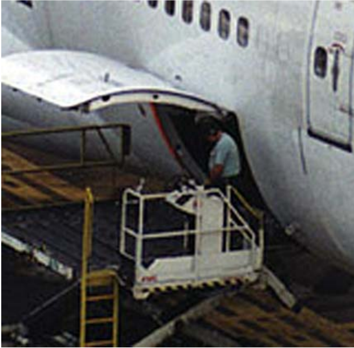
Caption for above photograph: Closeup of open forward cargo door showing open manual locking handle, several of the bottom eight latches, forward leading edge midspan latch, and the aft leading edge midspan latch pin.
