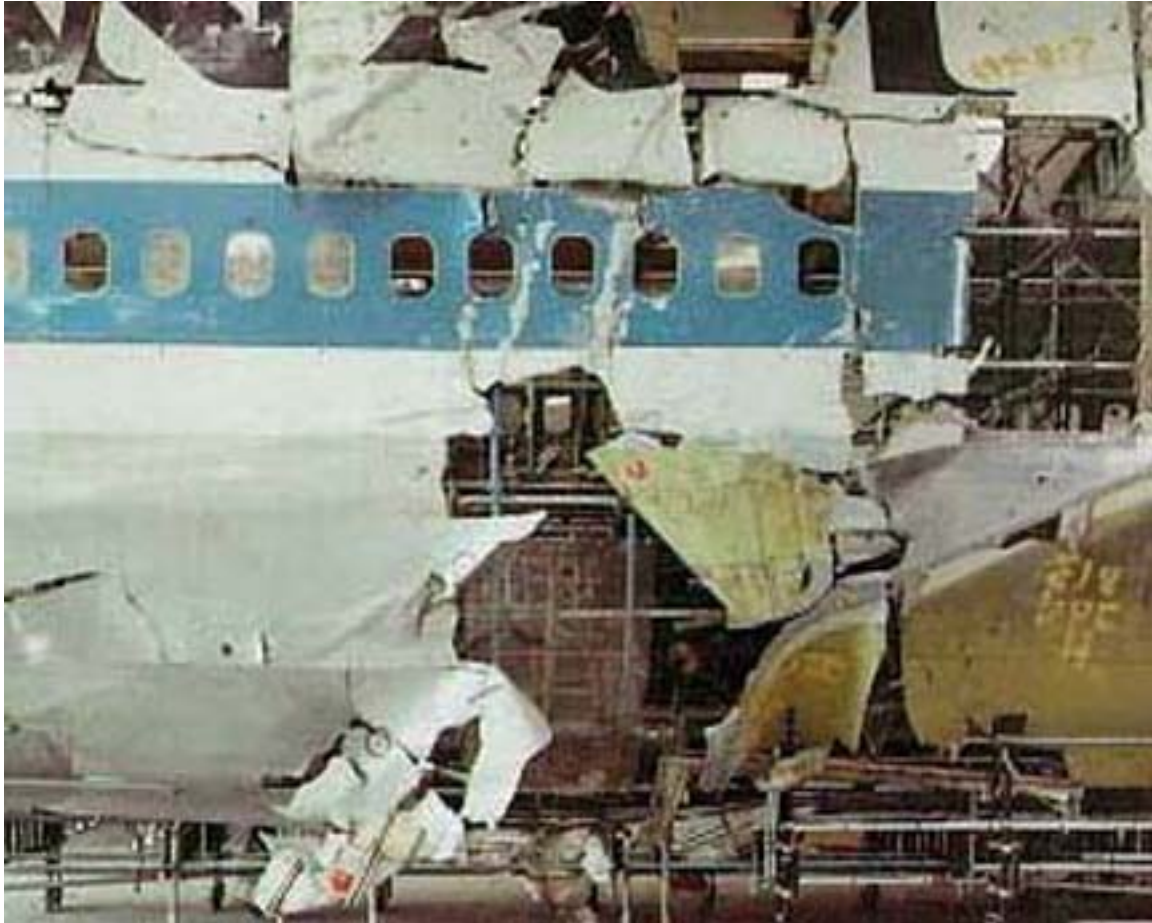
Caption for above photograph: Port side of Pan Am Flight 103 forward of the wing showing the small 'bomb' hole and relatively smooth and intact fuselage skin around it.
