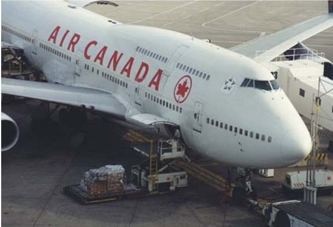
Caption for above photograph: Boeing 747 on ground loading cargo through opening outward nonplug forward cargo door. The tiny dot of the one midspan latch on the leading edge of the door can be seen.
