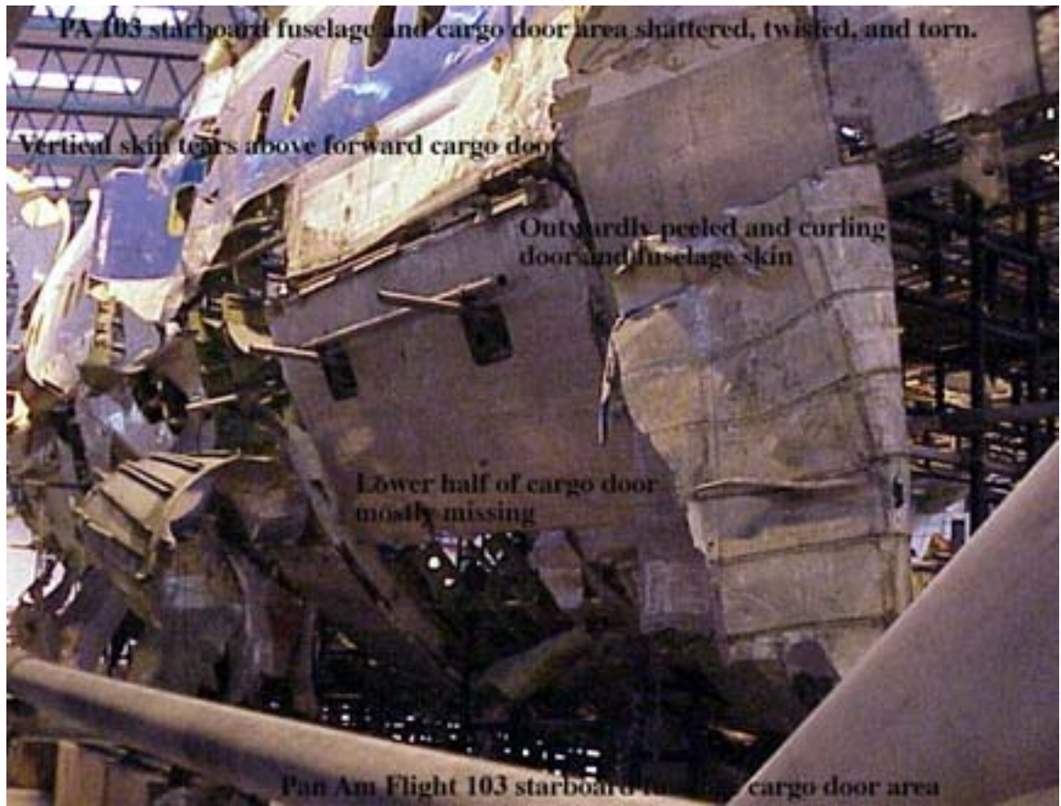
Caption for above photograph: Photograph from AAIB showing Pan Am Flight 103 forward cargo door area revealing the vertical torn skin above door, peeled back skin from the aft midspan latch, generally shattered area, and mostly missing lower half of door which includes the manual locking handle and the eight bottom latches.
